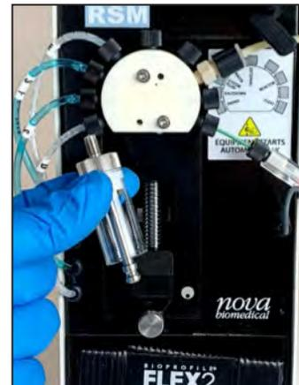
Figure 5.4 Remove Syringe Assembly
