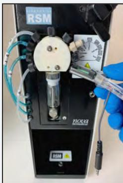
Figure 3.25 Tighten Air Detector
