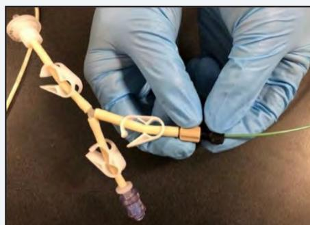
Figure 3.47 Adapter (left) and Reactor Line (right)
