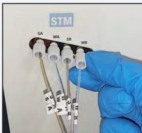
Figure 5.7 Sample Inlets and Outlets
