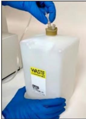
Figure 5.16 Luer Connection on Cap
