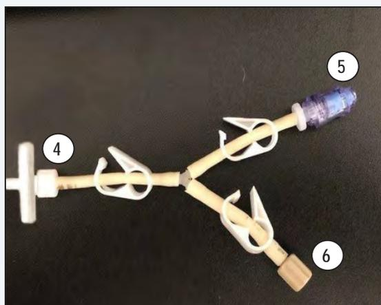
Figure 3.46 Reactor Line Adapter with Filter: (4) Vessel End, (5) Auxiliary Manual Sampling Port, and (6) Reactor Line End
