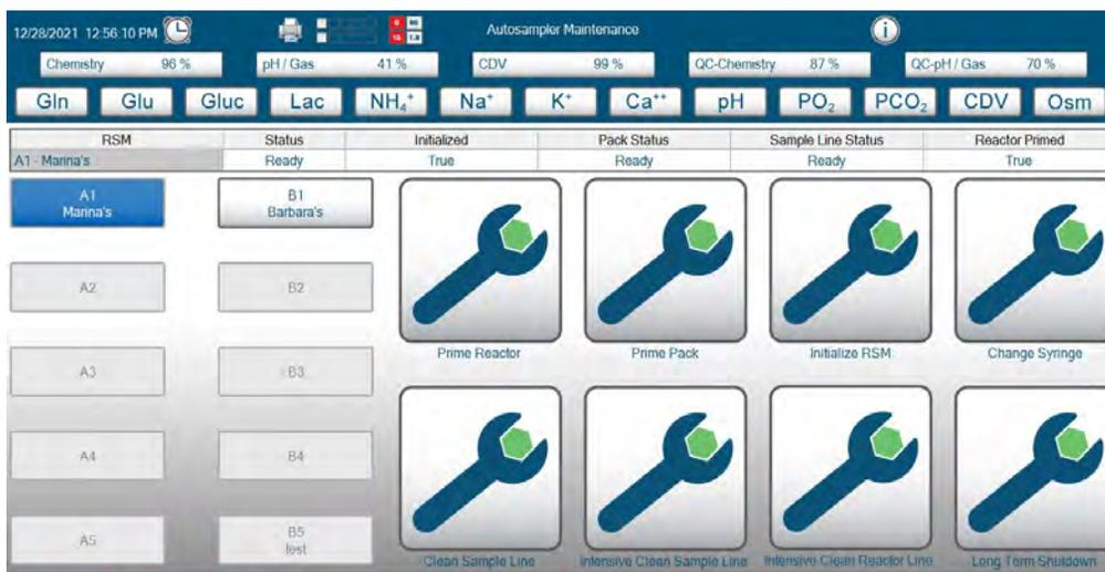
Figure 5.1 FLEX2 Autosampler Maintenance menu screen
