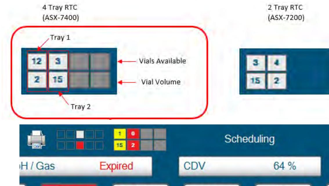
Figure 2.12 Retain Collector Status Indicator
