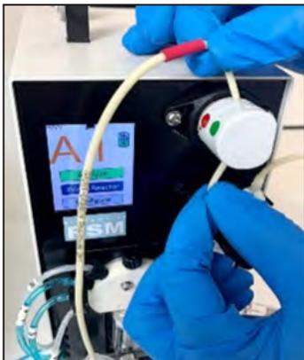
Figure 5.30 Vent Line in Pinch Valve
