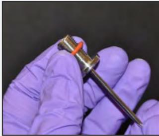
Figure 3.35 O-Ring on Threaded Dip Tube
