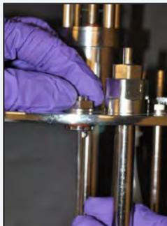
Figure 3.37 Threaded Dip Tube on Headplate
