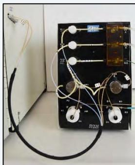
Figure 3.14 STM Tubing Harness Installed
