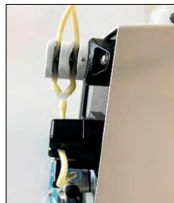
Figure 5.36 Reactor Line Y-fitting
