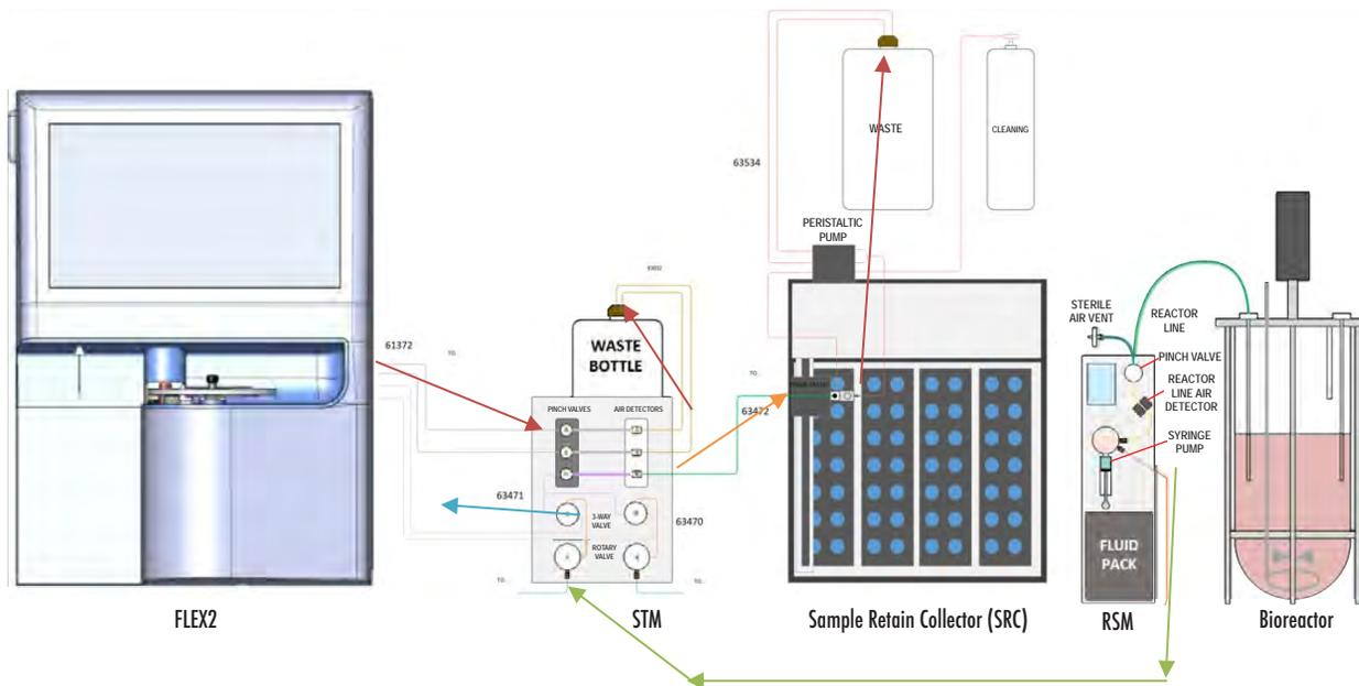
Figure 2.20 Sample Retain Collector Flow Overview
