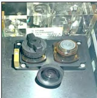
Figure 3.32 Cap B Removed to Show Septa
