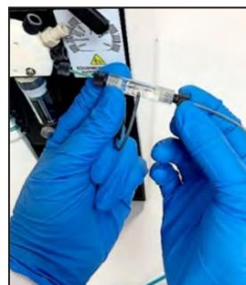
Figure 5.25 Sample Line and Sample Line Air Detector
