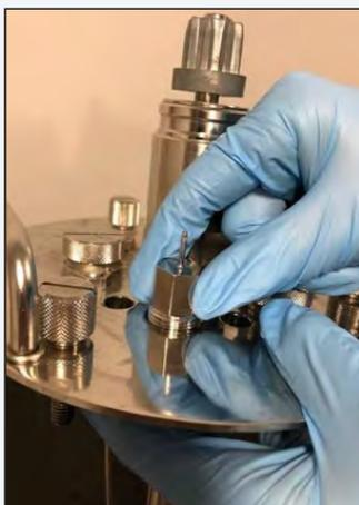
Figure 3.40 Dip Tube on Headplate
