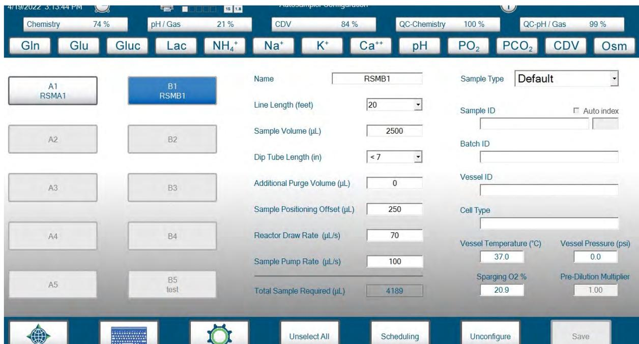
Figure 4.1 RSM Configuration menu screen
