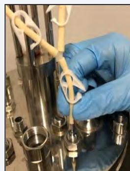
Figure 3.49 Adapter on Barbed Dip Tube
