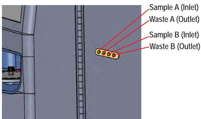
Figure 2.7 OLS Interface Ports (Right FLEX2 Cover)
