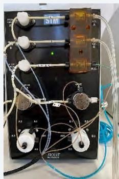
Figure 3.19 Waste Tubing Harness Installed on Nova Bottle
