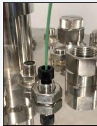
Figure 3.44 Reactor Line Tightened
