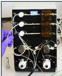
Figure 5.13 RC AD tubing in Pinch Valve
