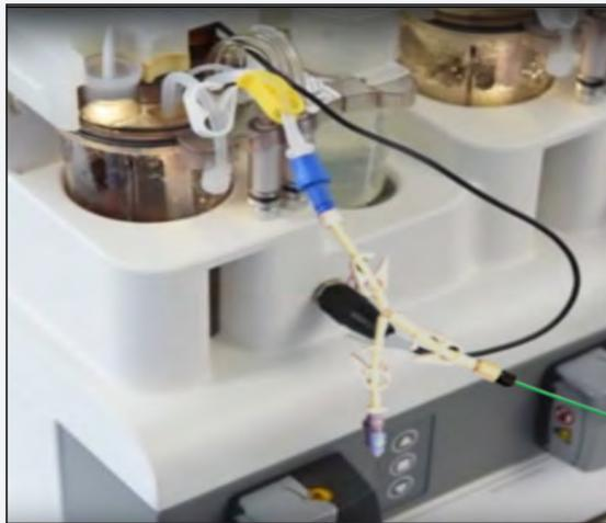
Figure 3.54 Reactor Line Adapter on ambr® 250 Modular Bioreactor Vessel
