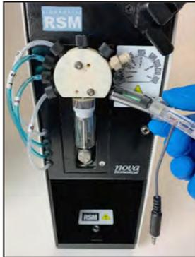
Figure 5.27 Tighten Air Detector
