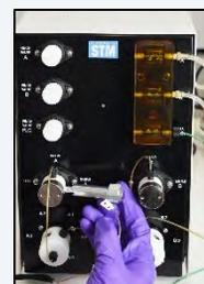
Figure 3.7 Sample Inlet A (VA)
