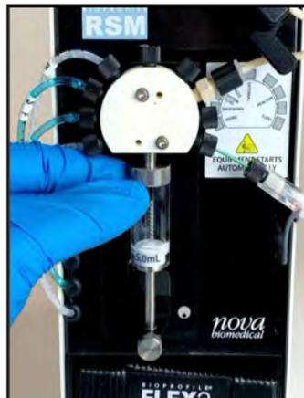
Figure 5.3 Unthread Syringe Barrel
