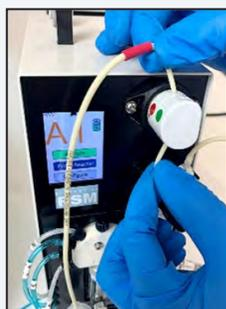
Figure 3.55 Vent Line in Pinch Valve
