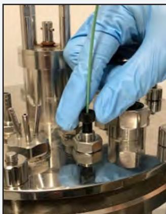
Figure 3.43 Threaded Headplate Connection
