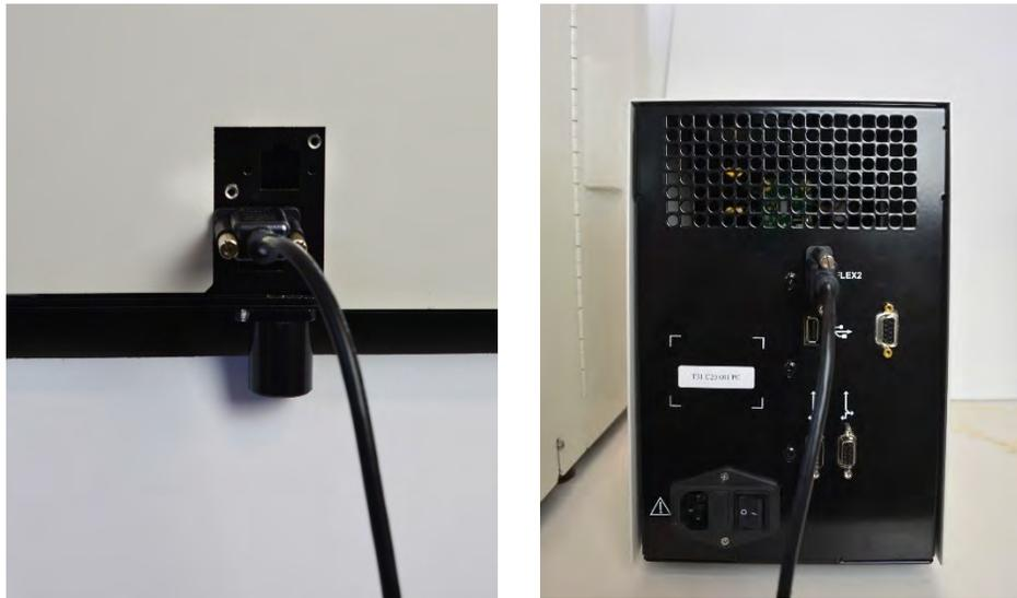
Figure 3.2 Designated rear COM ports for STM cable on FLEX2 (left) and STM (right)
