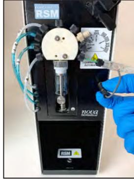
Figure 5.28 Air Detector Cable Jack
