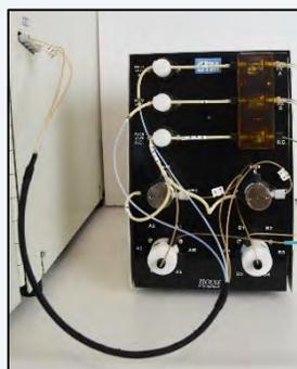
Figure 5.15 STM Tubing Harness Installed
