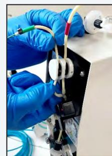
Figure 3.57 Reactor Line in Pinch Valve
