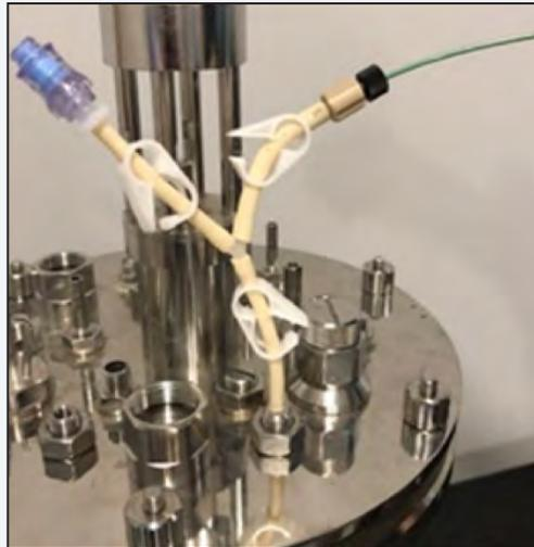
Figure 3.50 Reactor Line Adapter on Barbed Dip Tube Assembly
