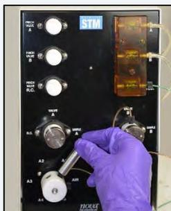
Figure 3.22 Sample Line on Rotary Valve A
