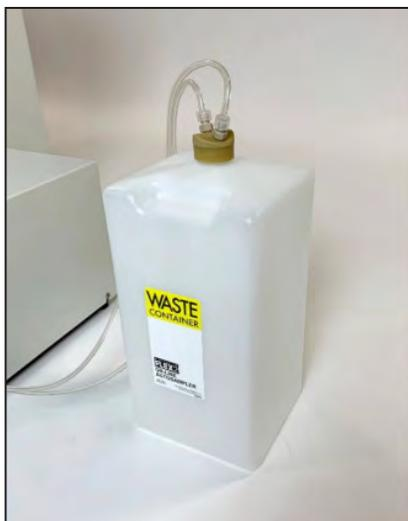
Figure 5.37 Nova OLS Waste Bottle with Waste Tubing Harness Installed
