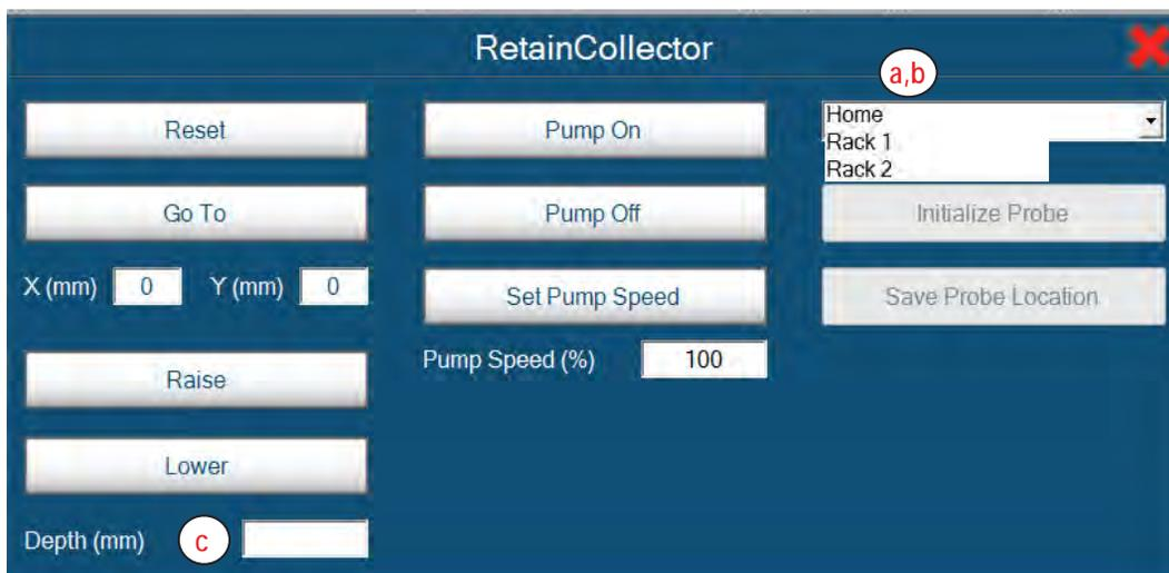
Figure 4.11 Retain Collector Probe Calibration Screen
