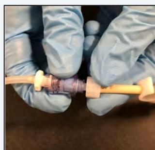
Figure 3.53 Existing reactor Manual Sampling Port (Left) and Reactor Line Adapter (Right)
