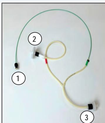
Figure 3.42 Reactor Line Assembly Segments: (1) Vessel End, (2) Air Vent Line, and (3) RSM End.
