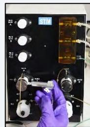
Figure 5.8 Sample Inlet A (VA)
