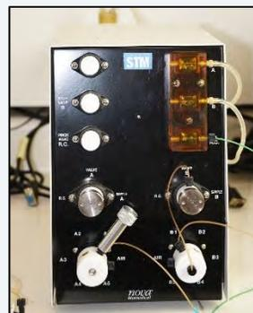
Figure 3.23 Rotary Valve A
