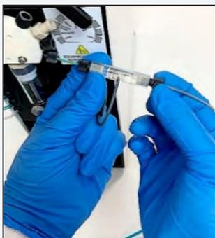
Figure 3.27 Sample Line and Sample Line Air Detector
