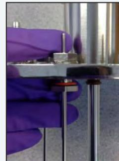
Figure 3.38 Barbed Dip Tube on Headplate.
