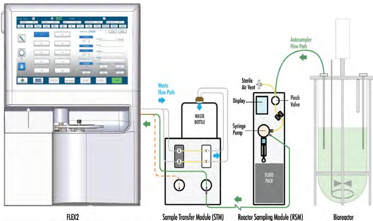
Figure 2.19 FLEX2 On-Line Autosampler Flow Overview
