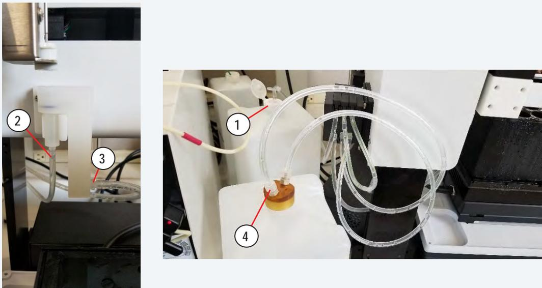
Figure 3.67 Wash Station and Wash/Waste Bottles
