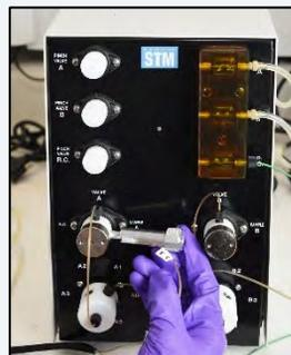
Figure 5.12 3-Way Valve A Bank to RC AD
