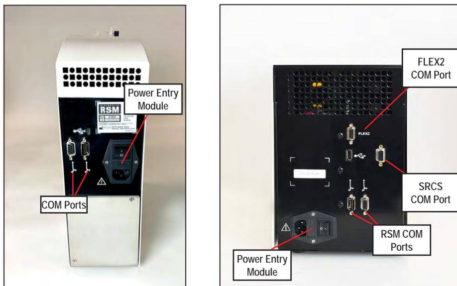
Figure 3.1 System Component Rear View- RSM (left) and STM (right)
