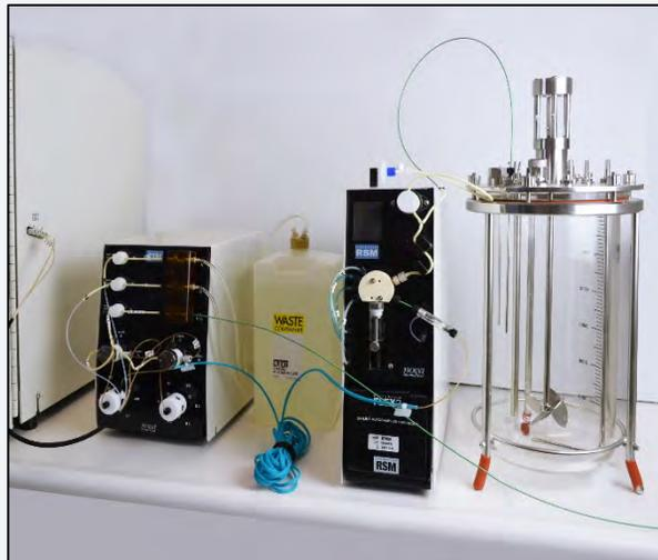
Figure 3.62 Reactor Line Fully Installed on RSM and Bioreactor
