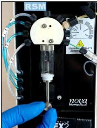
Figure 5.2 Bottom Thumb Screw
