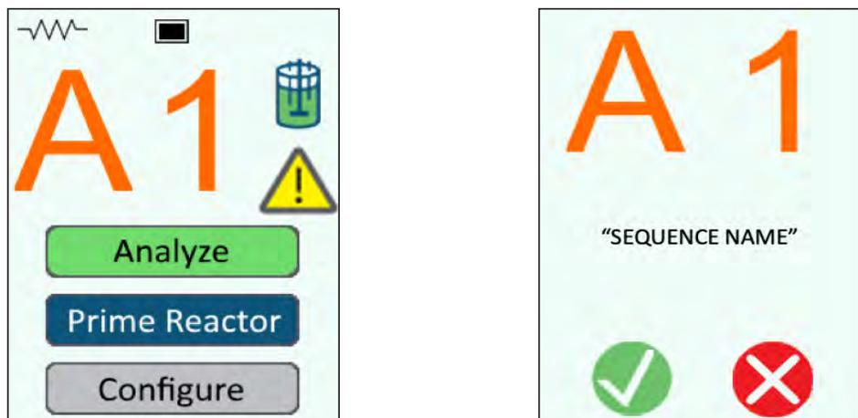
Figure 2.4 RSM User Interface Home Screen (Left) and Confirmation Screen (Right)
