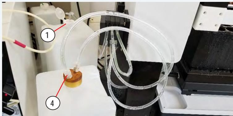
Figure 5.23 Wash Station and Wash/Waste Bottles
