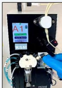
Figure 3.59 Reactor Port Luer Fitting
