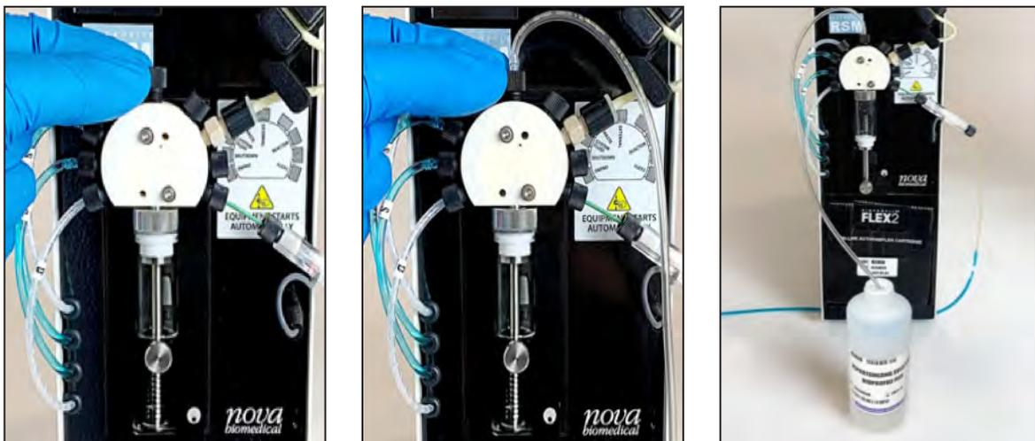
Figure 5.5 Installing the External Cleaning Line
