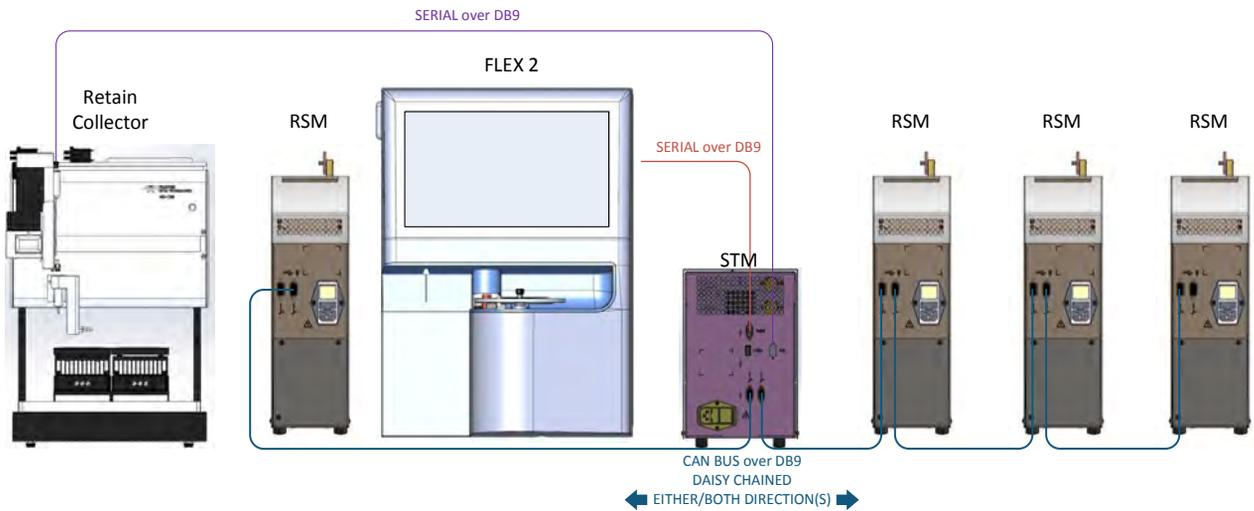
Figure 3.4 RSM COM cable daisy chain configuration
