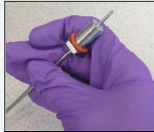
Figure 3.36 O-Ring on Barbed Dip Tube
