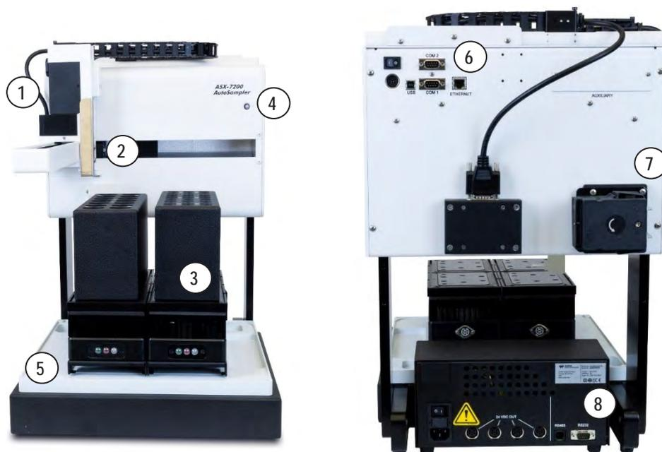
Figure 2.6 Sample Retain Collector Front/Rear View
