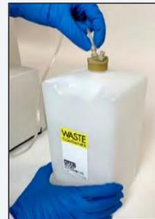
Figure 3.18 Luer Connection on Cap
