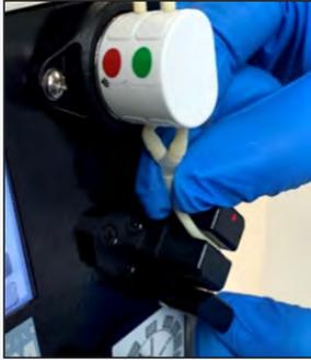
Figure 3.60 RSM Air Detector
